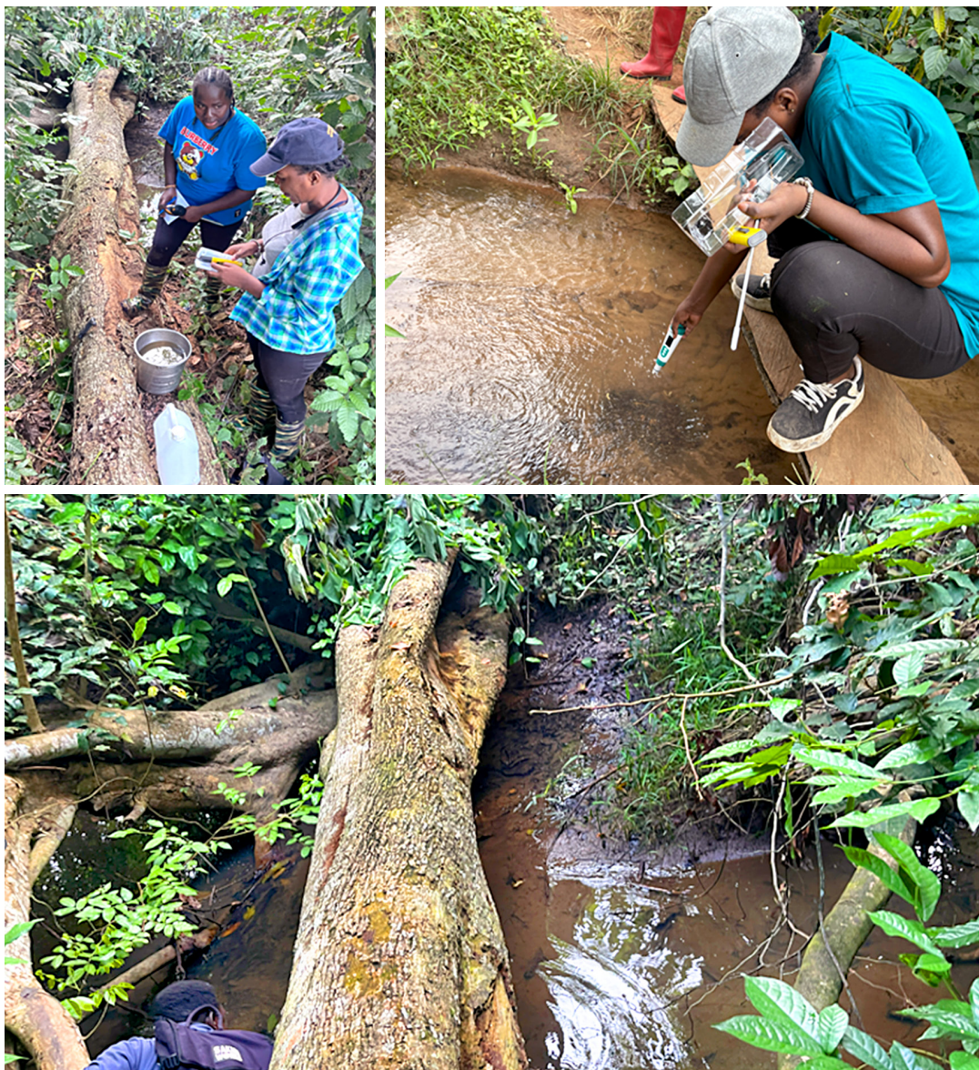
Figure 7: Testing water near cocoa farms for key physico-chemical parameters that might be impacted by agricultural practices.
