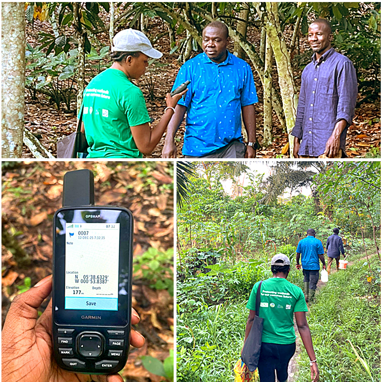
Figure 8: Using a handheld GPS receiver to spatially map the borders of cocoa farms for land use change analysis.
